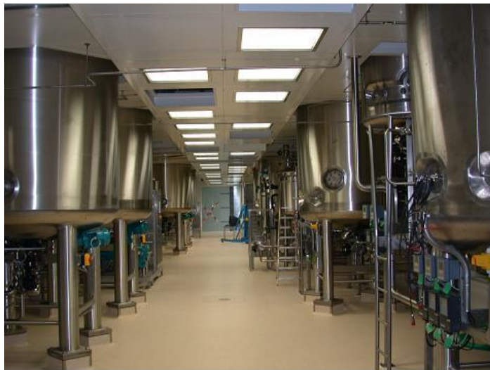
Large scale fermenters for virus production
